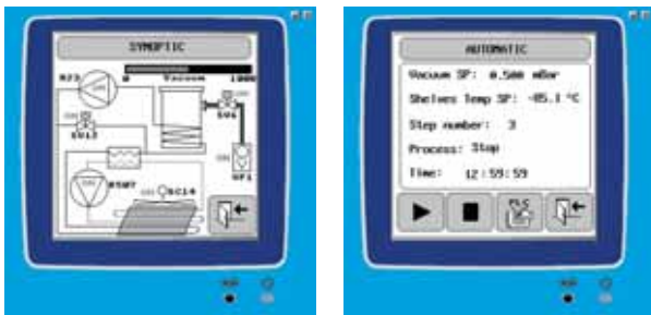
LyoAlfa 10/15 control panel screens
