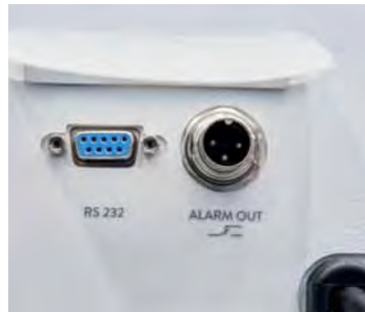
Standard-issue RS 232 interface and alarm contact
