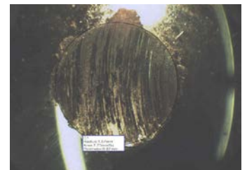
› Image capture of scar using Microscope with Digital Camera (19750-3)
